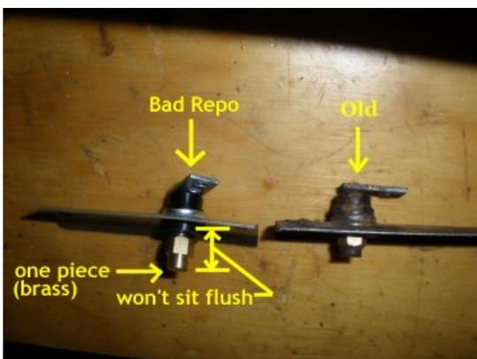
REPO Contact Brush (left) is a new repo, and (right) is the original. Couple problems with the new repo. 1) it does not seat flush, at least 1/8in off (requiring grinding down) 2) One piece, Brass will wear faster than a copper one.
