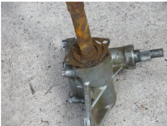
Loosen the upper housing clamp and pull up the tube, then unscrew the 3 bolts holding the upper housing cover. You should be able to pull the tube up off the steering column.
