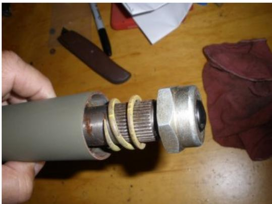
Now install the steering wheel spring and the steering nut with horn button so that the wire and contact do not get bent up.
