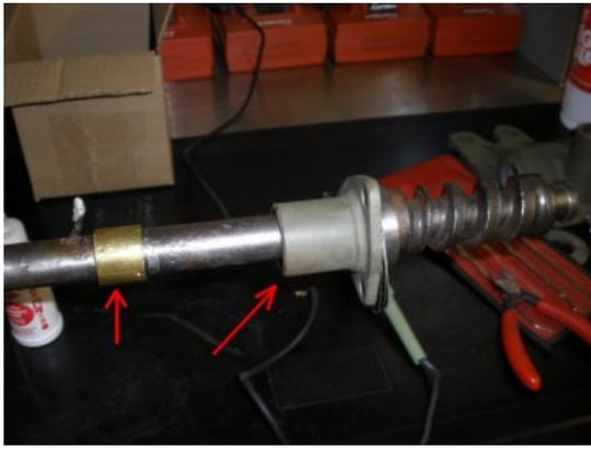
\*check\* make sure you have your top CUP and HOUSING TOP COVER (and shims) prior to soldering... make it a lot easier for fitting. Add Flux to surface area and wire prior to soldering otherwise solder will not stick. Place wire on copper bushing and solder on top of wire until it melts to bushing
