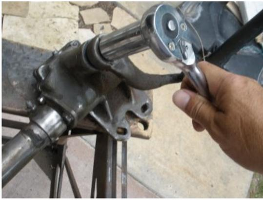
After knocking off most of the crud with a wire wheel on a grinder, we remove the Steering Gear arm nut. In order to clean further, we need to pull off the arm.
