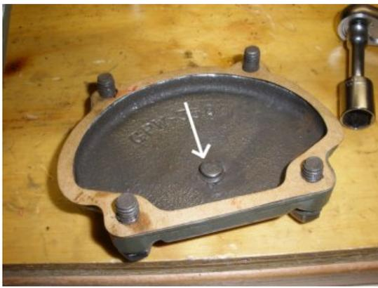
The housing plate screw will allow the sector shaft to move back to a certain point in the housing. If you adjust this to far in, the shaft will become to tight, if it is to loose, the teeth may skip in the worm gear. Note: here you are preparing to install the copper washers. It is a good idea, to heat red hot, and cool in water, the copper is annealed and all previous stresses from tightening are relieved
