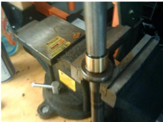
Next, to install the contact bushing you will need a soft piece of wood, a washer or the old cup. In a vise, we used the old cup, and sprayed WD40 on the shaft where the bushing is started. With the wood block at the top of the shaft gear, we start tapping the shaft downward. Because the inside piece is plastic, make sure you have plenty of lubrication in the process. Continue all the way down the shaft into position.
