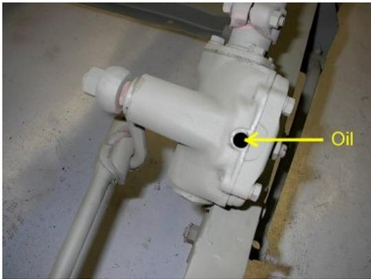
Once you install the Steering column on your frame, remove the plug and add your oil and fill the housing to the top.
