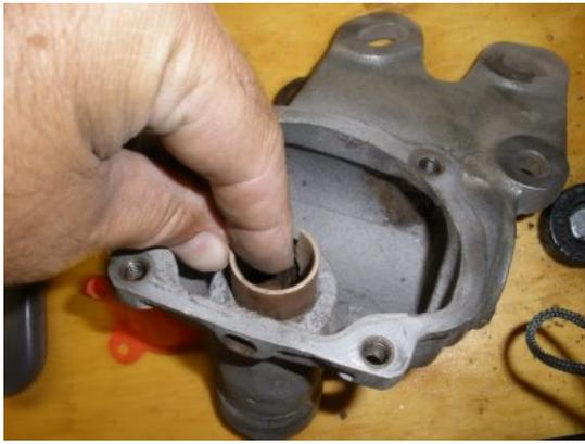
Once the bushings broke down a bit, they were easy to pull right out.
