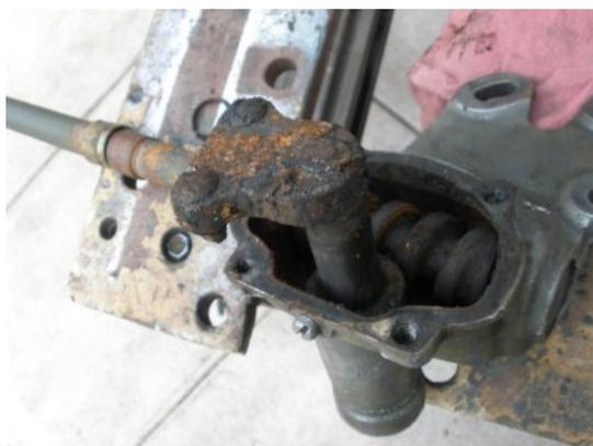
By rotating the steering column, you will see the lever shaft start to force itself upward. You can pull this out with your hand, or wedge a screwdriver in and finish bringing it out.
