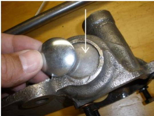
Punch out the housing plug. Here you see it with the replacement plug. Turn the housing over and the plug will punch right out.
