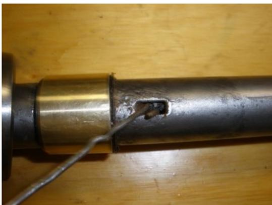
When you pull the wire back and you get to the opening in the shaft it is going to be very tight. You need to twist the pull wire while pulling about 90 degrees before the wire will fit through the opening.
