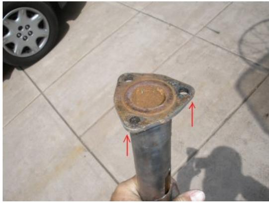
With a rubber hammer, tap the upper housing cover off the tube. This should separate easily.
