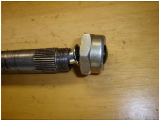
Temporarily install your horn nut and horn button on the top of the shaft; this will keep the horn wiring from catching on things as you work with the shaft.
