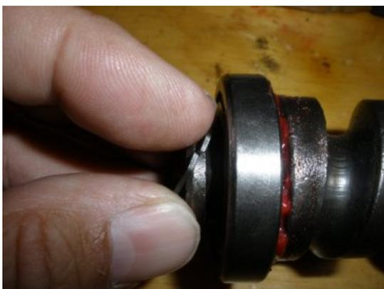
Press one side of the ring around the ridge on the worm gear and press the ring around the ridge and it will snap into place. This side is the easier of the two.
