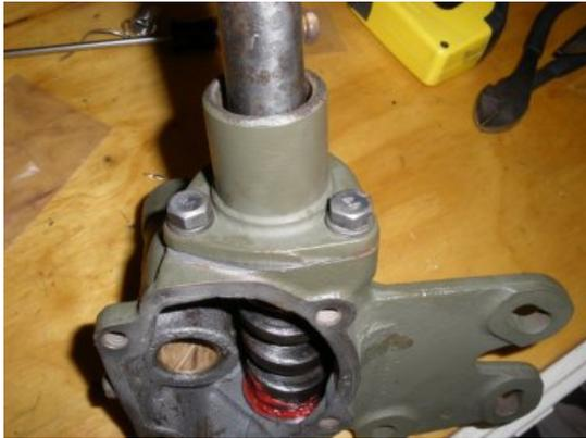
Now install your main shaft cover tightening the bolts down. When tightened, turn the main shaft and tug up and down. If you have play up and down, then you need to take a shim out, if turning is really tight, then add a shim. In this case, it was a little loose with play in the top and bottom.
