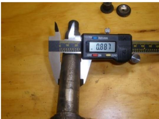
Last, measure the shaft as well. This should be within a .001 value to the inside diameter of the bushings.
