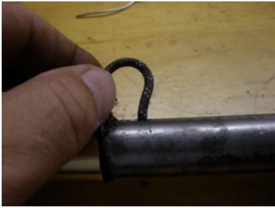
You want to pull the excess wire through with just a little extra at the top of the shaft. If you don't, you will have some back pressure from the wire when you try and apply the nut.
