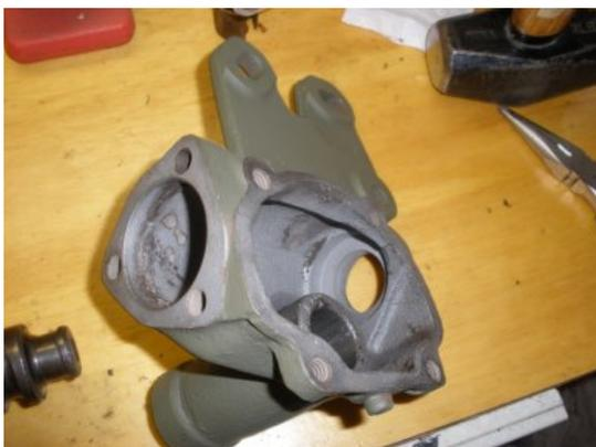
Now that the housing is primed and painted you can start to assembly the rest of the housing.
