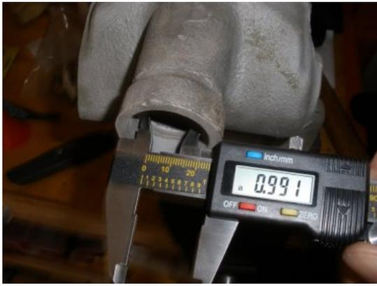
Prior to installing your replacement bushings, measure the inside diameter of the housing, and the outside diameter of the bushings. The bushings should fit tight, but the tighter they are, the smaller the inside diameter of the bushings will become when pressed in.
