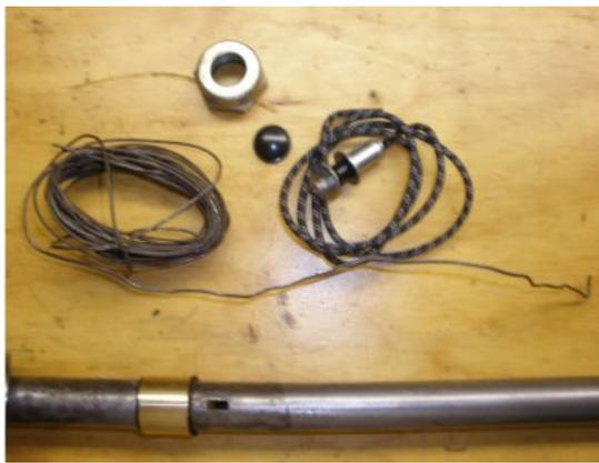
With the contact bushing down in place, lets prepare to install the wiring for the horn. Here you can see you will need some wire to pull it through. You might want to have your horn nut handy as well. You can install the top to keep the horn connector from catching on stuff prior to installing on your jeep.
