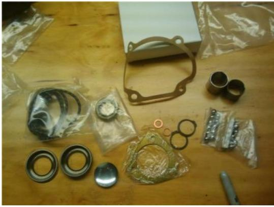
Here you see the gear box part kit, the horn wiring kit. This cost about \$100 from Ron, but the steering is very important in your restore, so it is recommended to replace all these parts.
