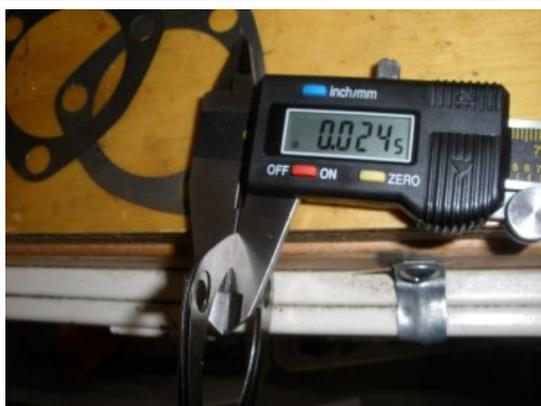
At this point you are ready to install the main shaft into the housing. Here I take out the shims and measure the .024 thickness that the TM suggests. when you install the shaft in the housing if it is loose (tugging up and down) then you have to many shims, if very tight in turning, then you don't have enough shims.
