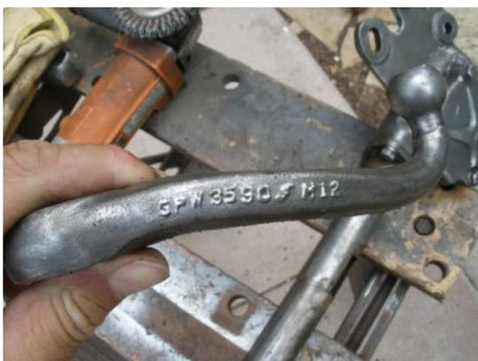
Ford OwnersThe steering gear arm will be marked with a GPW part number as shown here.
