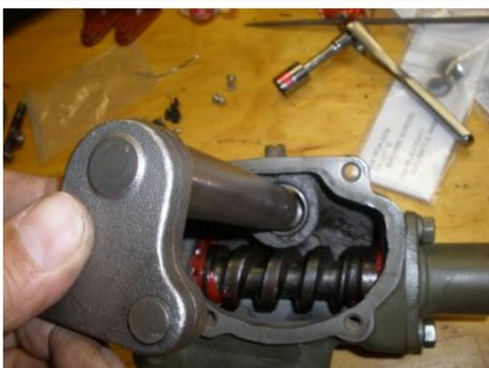
Now, insert the new sector shaft into the housing with the new bushings. In this case, the fit was too tight for the second bushing, so we needed to hone it out a bit to get it to fit through.
