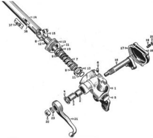
The Steering component in a WWII jeep is not very complicated. But, almost all restore projects have very old, probably rusting steering components that need to be looked at before you can drive safely. Here you see a breakdown of the steering box components from the TM-10-1513
