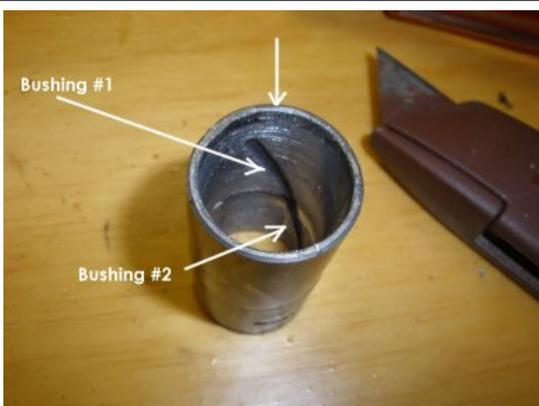
Take a look at your replacement bushings. From the replacement kit, you will see the short and long bushing together. Observe the groove in the middle. This is for lubrication flow on the shaft. The longer bushing groove stops before the edge so that the lubrication does not make it to the seal and leak.
