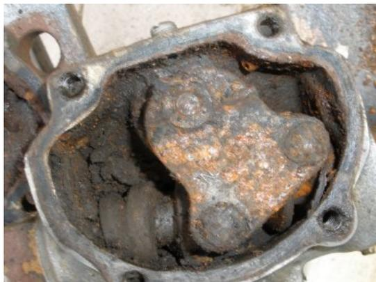
At a closer look inside the housing you see signs of rust around the lever shaft assembly. To clean out some of the crud, you should be able to turn your steering column and watch the lever shaft rotate.
