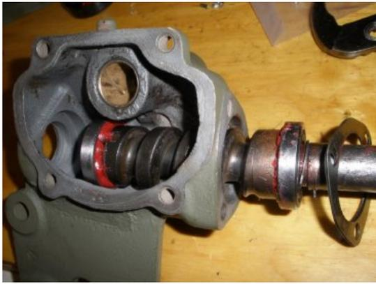
Run your shims up on the main shaft, and push your worm gear into the housing. It should be a little snug, but will fall into the housing by a firm press into position.
