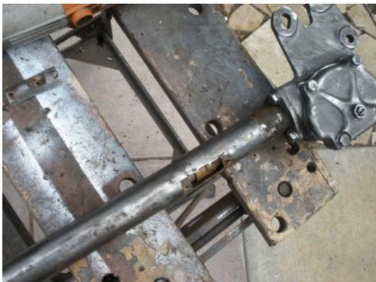
With the Steering gear arm off, we continue to wire wheel the steering column. Here you see the tube is cracked around the terminal for the horn connection.
