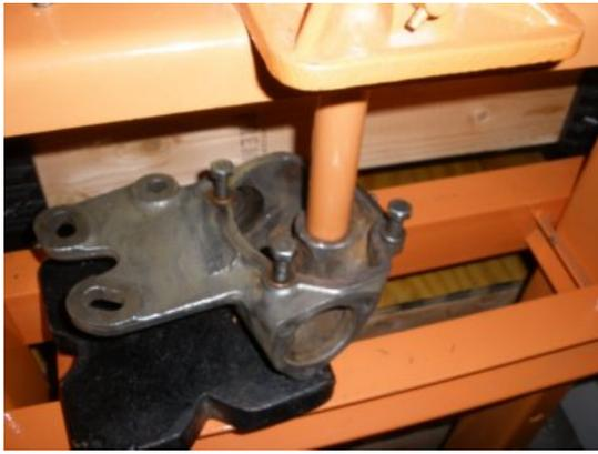
Next, press the bushings into the housing. You should line up the groove on the bushings so that the lubrication will flow to the shaft
