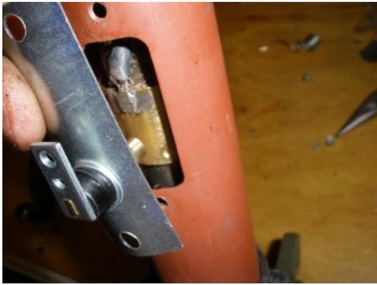
Here you see the contact will run on the bushing for the horn just fine. It lined up well and will not hit the soldering.
