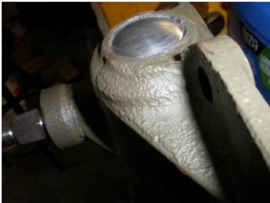
Next install the housing plug at the end of the housing. Clean your surface around this area and tap the plug into place.
