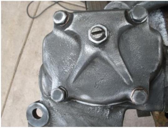
Here you see the side cover is cleaned off so we can prepare to remove it. Ford Owners Note the F mark on the side cover.
