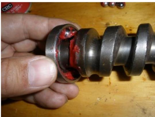
Start by installing the balls in the lower cup. Place some grease in the cup because the small ball bearings will slip out, and the grease will cause them to stick. Start with adding a couple balls, then press the cup on and put the rest of the balls in. Note: you can prep with all the balls because it will not fit over the retainer on the worm drive.
