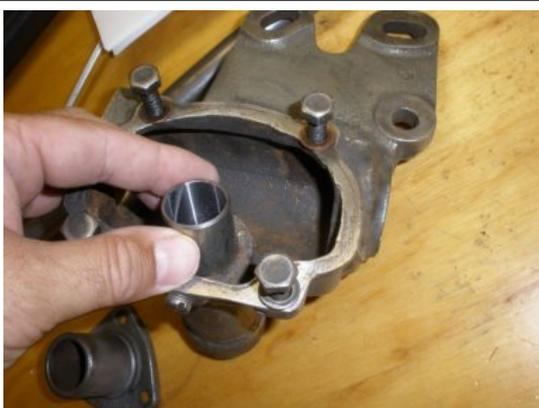
Next, line up the bushings to be pressed in. Here you see the bushing with the groove all the way to the end which will feed the lubrication to the shaft. You will want to line up the other bushing and press through the other side.
