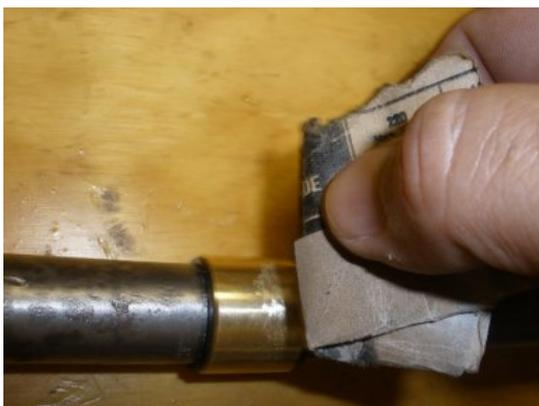
Next prepare the soldering area on the bushing by sanding the section that you will solder on. Note: the top of the bushing is where the contact will ride on the bushing from the steering column.
