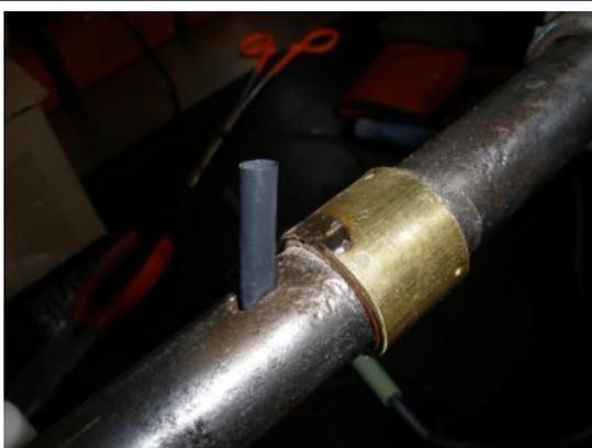
\*optional\* here we put a little extra protection on the wire with a little heat shrink wrap. When the wire is being moved around with steering, this will protect it around the hole it comes through. In addition, we prep the bushing with a little solder prior to bringing the wire down.
