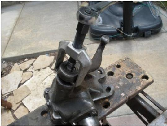
With an inexpensive puller, we pull the arm off. Note: don't try pounding this off as it will require a puller to do it correctly without damaging the arm.
