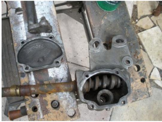
Cleaning the parts up a little better, we now are ready to press the steering column out of the housing and blast all of the parts.
