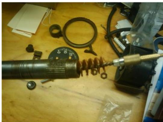
Next, check the inside of the shaft for rust. Here I used a 20 gauge gun cleaning brush and rod to clear out all the rust from the shaft.
