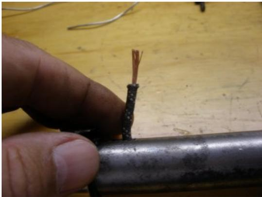
Prepare the wire to be soldered by cutting away about 1/4in of insulation. Place the wire over the bushing, and cut about 1/4 in below the bottom of the bushing. Then strip the wire and prepare for soldering.
