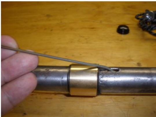
Run the wire down the steering shaft to top end. There we will hook it up and pull it back through.
