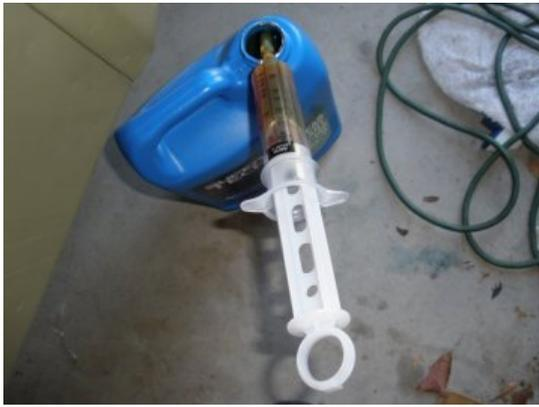
Now, use your SAE 90 wt oil and a device to pour into the top of the steering plug hole. Here you see a very inexpensive surenge that will allow us to insert the oil into the housing easily and without mess.
