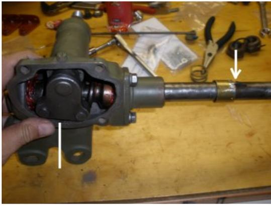
The sector shaft should push all the way through and line the teeth up on the worm shaft in the center. Here you see the contact ring is lined up in the middle of the shaft. If you have issues, you will want this lined up with straight wheels later.
