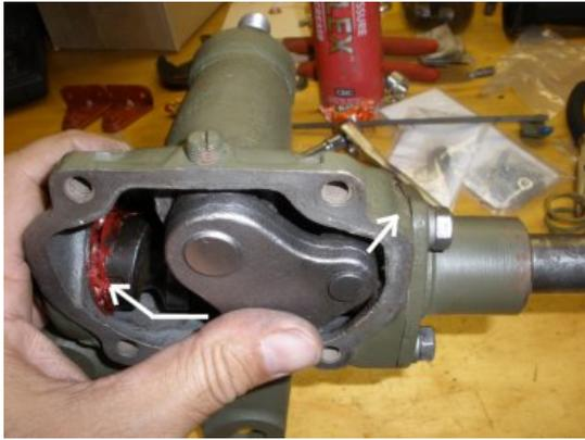
Once the sector shaft is in, turn the main core shaft and feel the sector shaft fit with the worm gear and verify that it is lined up in the middle where the contact wire is facing upward as mentioned before.
