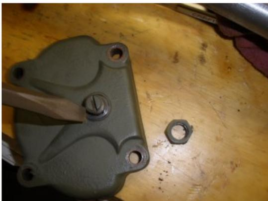
Before you replace the cover plate on the housing, you want to loosen up the screw on the housing plate. This screw keeps the sector shaft from pushing itself out of position when the worm shaft is moving. If it is on too tight, the sector shaft will not move.
