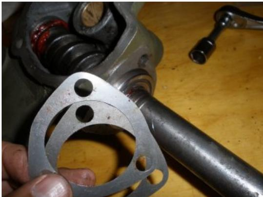
In this case, I needed to reduce the shims down to two (from three) to get a snug fit. It was about .018 measurement. Repeat the steps to put back on and test. Ahh, much better. Turns well with no play.
