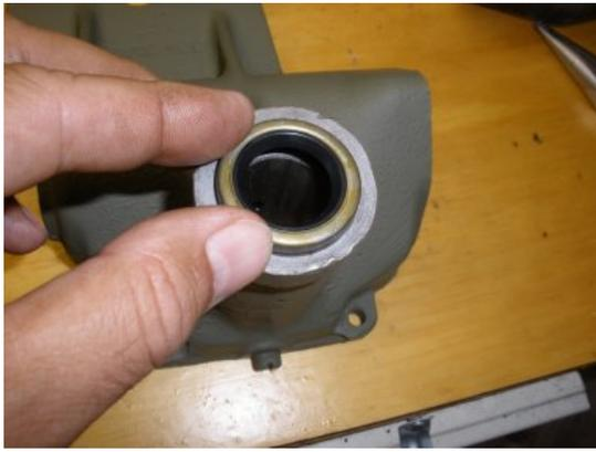
Here, install the housing seal by tapping it into the housing. It should be good and snug.
