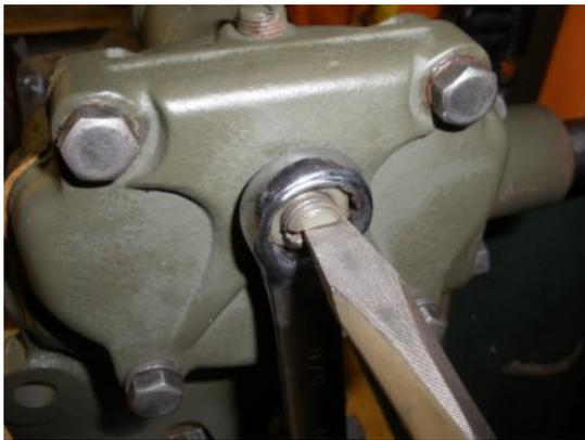
With the cover bolted on, rotate the cover screw clockwise while turning the main shaft. Turn until you feel a slight drag on the sector shaft while turning. Back off just a bit, and tighten the nut around the cover plate screw. Test the main shaft moving from one end to the other.
