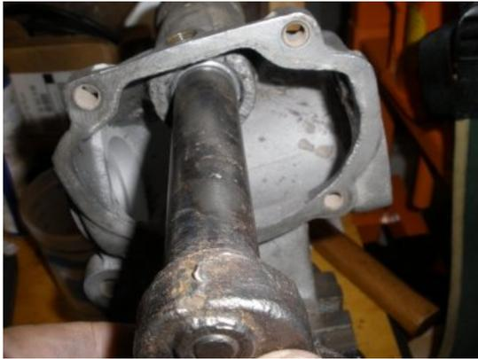
After you have the bushings pressed in, test the fit with the shaft. Anticipate this being very tight. If it is too tight hone out the bushings a bit so that the shaft will fit and rotate firmly.
