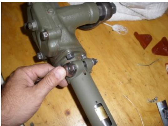
Now take the Shaft tubing and tighten it to the housing. Align the the contact bush opening with the top of the housing. If you don't it will be hard to reach when your wire up your tub.
