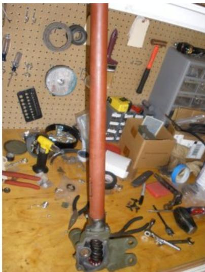
Install the main tube over the main shaft. Here, check two things. First the turning of the main shaft that there is no drag, and second look to see if you contact area for the horn is lined up. Note the position of the contact area hole. Should be pointing upward for the connection to the horn after you install the steering.
