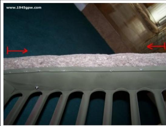
I stapled the ends of the complete felt piece first, then worked into the middle. This helps the felt stay in place and keeps it from buckling in between staples. Once you get a couple of them in, it starts to go pretty fast.
