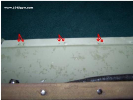
My impression of installing radiator felt was much different that what the actual effort needed. I thought simple, push staples through felt and clamp down. I also thought I could do this with the grill on the frame. Wrong. You will need, large pliers, Needle nose pliers, and an Ice pick or nail. Unless you have a repo grill, your staple holes should be present on your grill.
