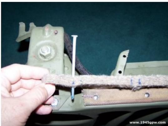
You can use an Ice pick or a long nail to poke holes into the felt. I didn't have an ice pick, so I used a large nail and pushed the nail through. Lay the felt up on the grill and see where it should align with the markings and place your nail on that spot and push through. Make sure you have it lined up straight across the grill shroud. The felt is really thick so this takes some doing.
