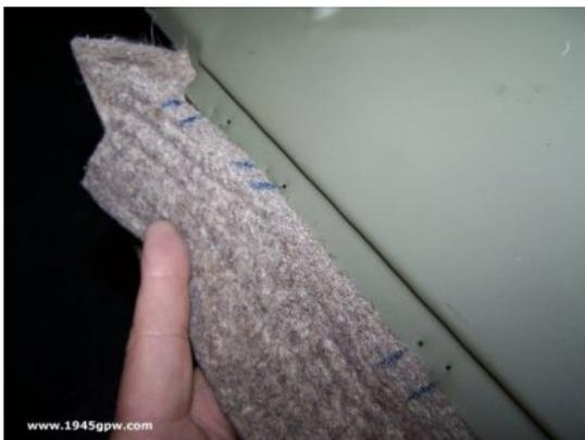
Since the felt does not have predrilled holes you will need to line up your pieces and mark where your holes should line up. My guess is that every jeep is different, so you will need to mark each hole as shown.
