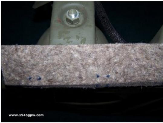
After each hole was created, I marked it with a felt pen. After you create the hole it is hard to find it.... so I marked the hole so I know where to place the staple when needed.
