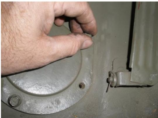
Install your master cylinder cap, and floor cover, and you are almost completed.
