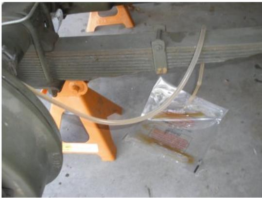
Now with all the speedbleeders now in the wheel cylinders and tightened down, move back to the Rear passenger side, and attach the tube retainer in the line. Loosen the speedbleeder about 1/4 - 1/2 a turn. Pump the brakes slowly about 4 times. The speedbleeders will open pushing the brake fluid out, and close when the pedal is retreating. Here you see the line is full and the fluid being push out with each brake stroke.
