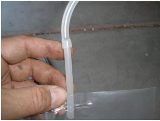
Connect the tube to the retainer bag. Now you are ready to start removing the old bleeders and replacing with the new speedbleeders.
