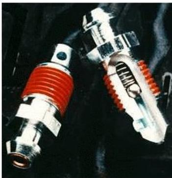
In this article we are introducing SpeedBleeders. No vacuum pump, very simple, one person method using by using [www.speedbleeder.com](http://www.speedbleeder.com) Speed Bleeders. If you look at the picture, you see how speed bleeders work. With the bleeder open a 1/4 turn, and tube connected to the bleeder, a hobbyist can push slowly on the brakes, pushing fluid out, but when your pedal comes up, a check valve will stop air from entering the system.
