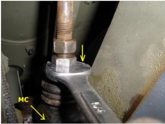
**Check the foot pedal** Now all of your brakes should be adjusted, the last adjustment is back on the master cylinder armature. Push in your brake pedal and check to see if it goes down and gets tight about 60% down. If so, you are at a good spot, no other adjustments needed.
