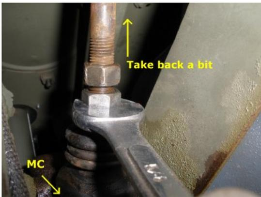
After installation of the speedbleeders you might find that your brake pedal goes to the floor. If so, you need to adjust your brakes now that all the air is out of the lines.
