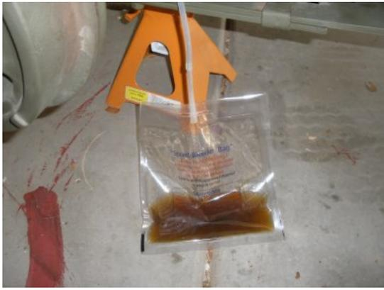
I moved to, and finished the passenger side front wheel and I was looking at the amount of fluid I now had in the retainer bag. At this point you want to check your master cylinder fluid level. I added more fluid to the master cylinder because you don't want the cylinder to go dry and get air back in your lines.
