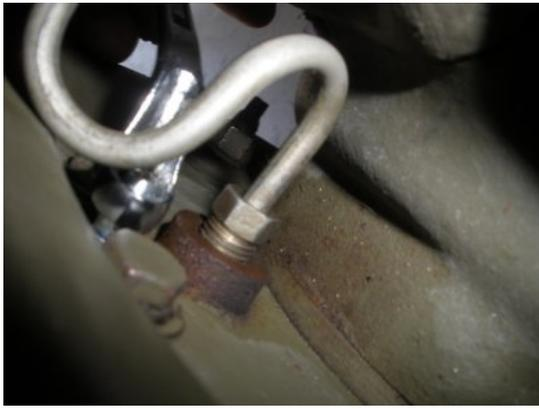
Repeat this process for the other Rear wheel bleeder on the driverside. You will note that the fluid has no more pressure, so the leakage should be minimal.
