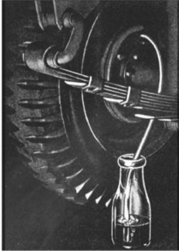
Bleeding brakes can sometimes be very frustrating. With hydraulic brakes you do not want any air in your lines. In most cases, it takes a two people to bleed brakes. One to open the bleeder screw, and the other to pump the brakes.
