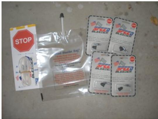
I used the SB1428 # 1/4 x 28 speed bleeder which are \$7 each, and the reusable retainer bag at \$3, and the reusable 1/4" tubing at \$3 (total \$34).
