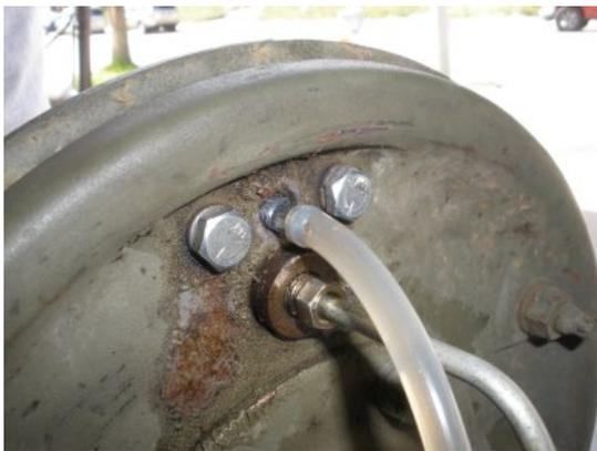
With a closer examination, you can see that the air in the fluid has already been pushed out. Now, tighten the bleeder (clockwise) and pinch the tube off at the bleeder and the fluid will flow down into the retainer bag.
