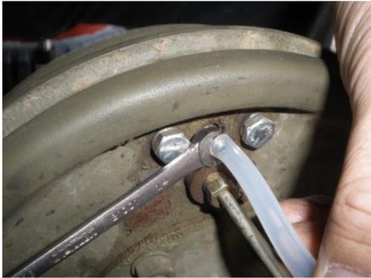
Starting with the Rear Passenger wheel, place the tube from the retainer bag over the existing bleeder and loosen. You should have a fair amount of pressure pushing the fluid out. Wait till the fluid has stopped, and loosen all the way out and remove.
