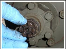
Once the cotter pin is removed, the axle nut should unscrew pretty easily.
