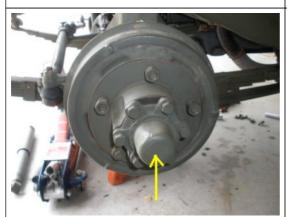
Start by removing the hub from the front axle. Very easy to wedge a screwdriver and pry the cap off.
