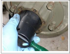
The bearing nut tool allows you to insert an object to help turn the nut if it is on there tight. Here you see a simple screwdriver was used to help turn.
