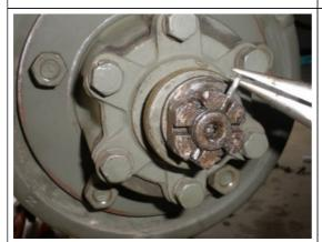
Next you will see a nut with a cotter pin. Straighten out the cotter pin and remove it.
