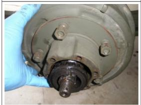
At this point the Brake drum is ready to be pulled off. Here, you see with a small tug, I pulled the drum out a bit, and you notice the <b>wheel bearings</b> are shown. The wheel bearings will drop out when you pull the drum off so be careful to catch them.
