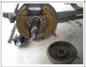
And you see the brake drum is now removed off the axle.
