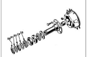
To remove the front brake drums require removing a few nuts, washers, bearings before the drum will come off. In particular, items 18-22 will be removed before the drum can be removed.
