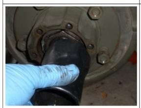
To remove the wheel bearing nut, use the large bearing nut tool to turn this nut. The tool can be found at most WWII Vendor locations
