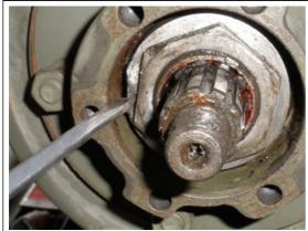
Next, you need to remove the wheel bearing nut. It is item 22 in the first picture above. Most likely the lock washer behind it has a bent lip. Use a screwdriver to flatten out the washer so the nut can turn.
