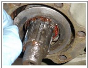
Once the first wheel bearing nut is removed, you need to remove the lock washer behind it. It will have a grove that goes into the axle, so you need to pull this out straight. Use a screwdriver and your fingers to help pull this item out.
