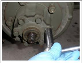
Next, remove the 6 nuts that hold on the flange. In some cases, the flange can be pulled off with your hands. Other cases, you may need a flange puller tool. Note: there most likely will be some shims behind the flange. Try not to damage them
