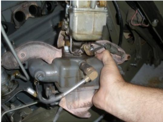
The Heat Control Valve is a neat piece of engineering for its time. To understand it, see the article on the Heat Control Valve detailed. Here we will show you what you need to do to replace the Heat Control Valve (sometimes called a Heat Riser). First you need to remove your exhaust manifold.
