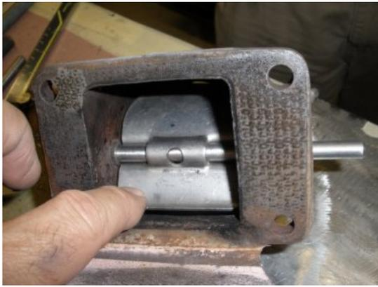
After installing the shaft see that it moves freely. We had to remove some burs in the bushing and we used some emery paper on the shaft to get it to move freely in the manifold.
