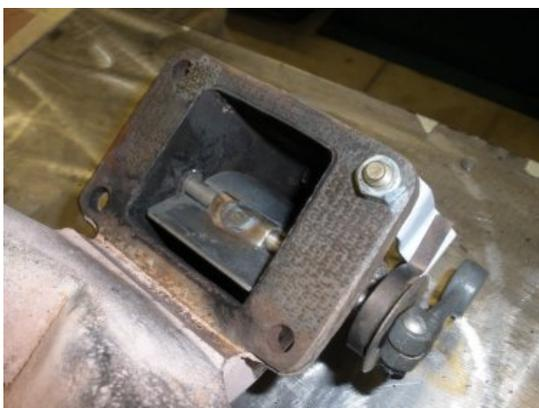
After testing this positioning, we welded the flap to the shaft. Note: be sure your welder is not too hot to warp the shaft.
