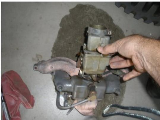
Separate the exhaust manifold from the intake manifold. (Four bolts on bottom). NOTE: Your Carburetor will probably still have fuel in it, so expect some spillage when handling it.
