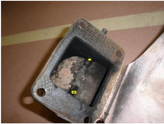
With my friend Harley (jeep is displayed on 1945mb.com) We plan to remove the center section of the flapper then heat the shafts and bushings on the side of the manifold and punch out. The yellow dots on the picture are where we punched a spot to drill the shaft out.
