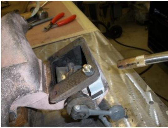
Completed, woo hoo! To test we hit the manifold with some heat, and watched the spring contract, and close the flap.
