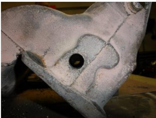
Now the manifold shaft hole is cleared out. REPEAT these steps for the otherside and remove the shaft and bushing as well.
