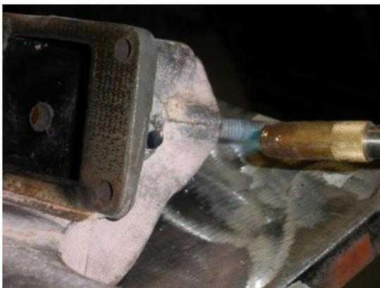
For a couple of minutes we hit one side of the manifold with heat on both the outside and inside of the shaft.
