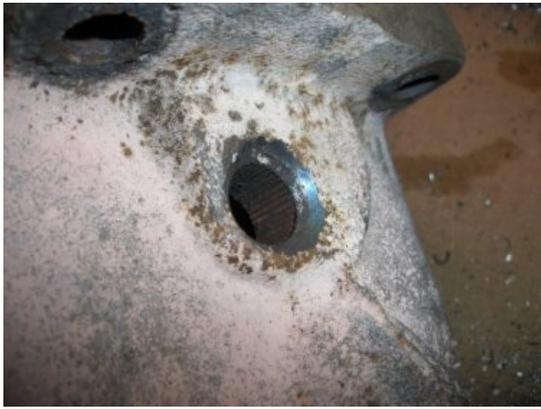
If you look closely into the manifold, the hole is grooved to hold the bushing in place.
