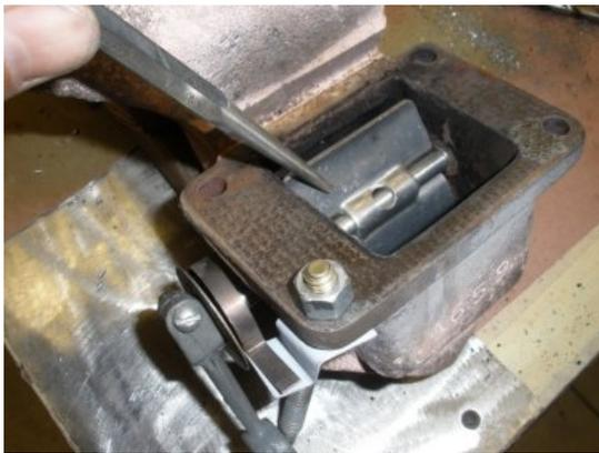
With everything in place, you will see that the flapper is loose. This will need to be welded into place. But first we want to make sure the position is correct. When the engine is cold the flapper should be open and gravity should have the arm pulled in a downward position. When the engine is warm, the arm will move up (from spring contracting) and the flap will shut close.
