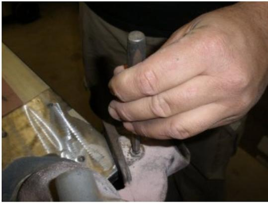
One side of the manifold heat control valve shaft hot, we took a large punch and punched the shaft out of the manifold. This should come out pretty easily.
