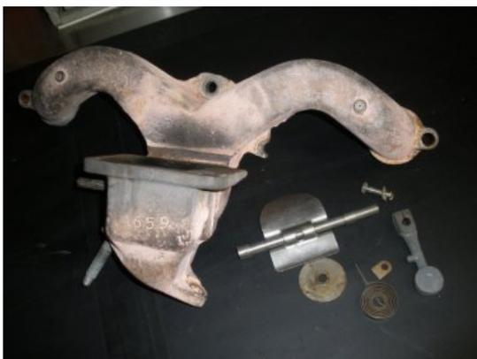
Here you see the parts needed to do the Heat Control Valve replacement. In this case, the current Heat Control valve is frozen in the exhaust manifold, so we need to remove it.
