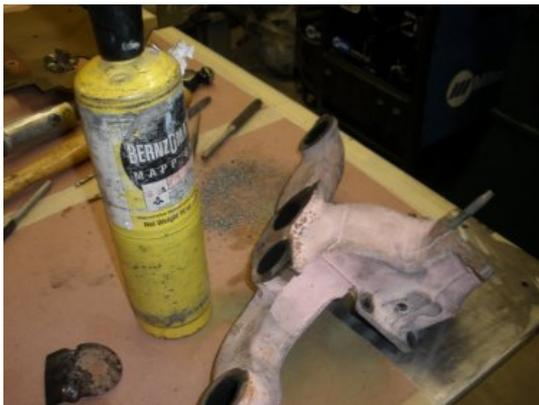
Here we use a little Mapp gas torch to heat the side of the manifold.
