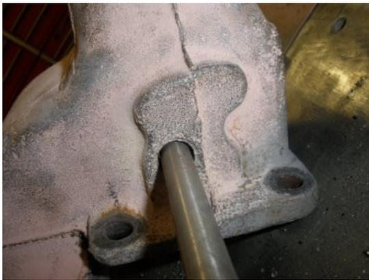
Now with the bushing hot, we used a larger punch and punched out the existing bushing.
