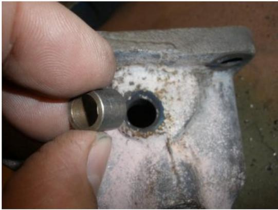
We measured the new bushing included in the kit and it was slightly bigger than the this hole we wanted to insert it into. So we heated up this hole again to have it expand a little before installing it.
