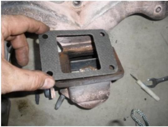
Add your manifold gasket and bolt on your four bolts back to the intake manifold.
