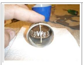
Screw the retainer on tight, and pull out of the container of lamp oil. Wipe off and you should see very little to no air in the glass bulb
