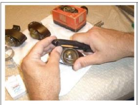
To remove the glass bulb can be done a couple of different ways. Use some sort of a knife to get underneath the glass lip and pull upward. Becareful not to damage the glass or the holder. Bulb should pop right out.
