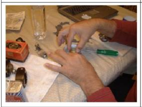
Next, submerge the glass bulb overflowing the glass bulb, then place the back plate in the glass bulb and screw on the retainer with the bulb completely submerged
