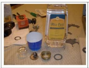
Now that the fix is made to the compass and the gasket is ready, I pour the non odor pure lamp oil into a cup I cut in half. I will submerge the entire glass bulb to remove as much air as possible.
