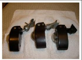
There are two different typs of hinges as shown. Two which have different arms and have a clamp style and the third is mounted to a surface via screws.
