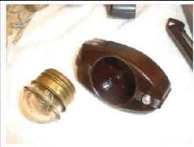
When the glass bulb pops out, you most likely will have some of the fluid all over the device from leakage.
