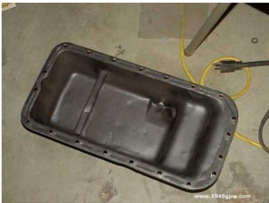
**DRAIN OIL:** This is optional, in my case, I drained it because I was replacing the rear main seal. So I removed the oil and the oil pan.
