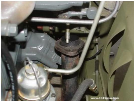
**DISCONNECT EXHAUST PIPE:** Remove these two bolts to the engine. Note: to get to these bolts, you will need to remove the horn
