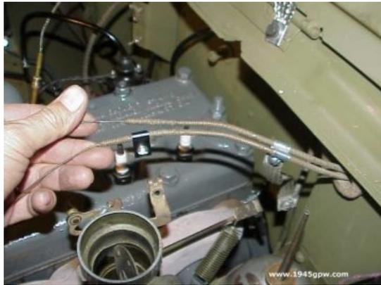
**DISCONNECT CHOKE/THROTTLE CABLES:** This cables comes from the firewall. Note, if you have a BOND STRAP from cables to Oil line, You should not have to remove it because it is connected to parts on the tub.
