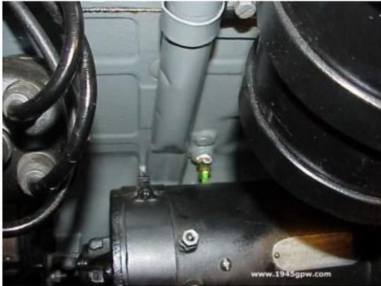
**DRAIN RADIATOR:** To start your engine removal, we start with draining the Radiator fluid from the block. While this is draining, continue with the other steps, as this will take about 20 minutes.
