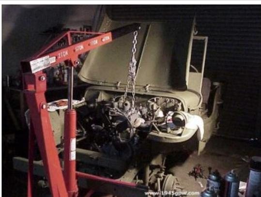
At this point, your bellhousing connection is ready to be disconnected. Be sure to have a jack under the bellhousing to support the weight as the engine is being pulled out the front. In my case, I will pull it out about 2 inches in order to allow the crank to drop and I can get the seal back on.
