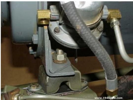
leave the engine mounts secured to the engine and unbolt them from the crossmember. It makes it a lot easier when reinstalling the engine because you don't have to line the mount studs up at the same time you're trying to line up the clutch splines. (tip from Pete Silfven)
