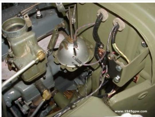
**REMOVE HORN** The horn will be in the way of you reaching the exhaust pipe and the oil line disconnect. Remove this and you will be able to reach these items.
