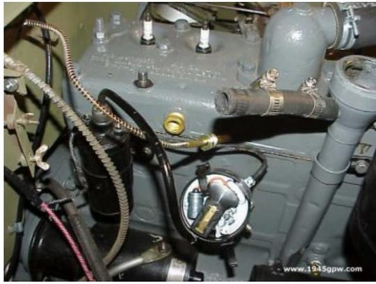
**DISCONNECT TEMPERATURE GAUGE:** Cable comes out of the firewall, so be sure this is removed from Head.
