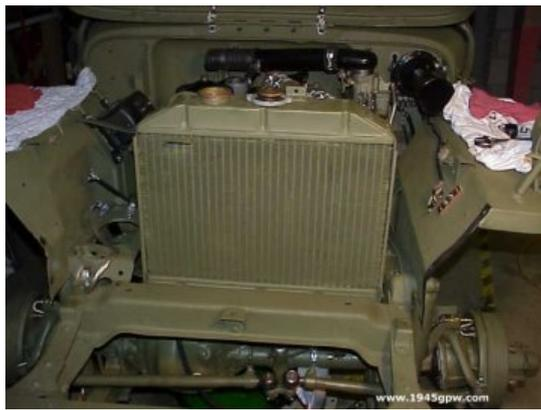
(OPTIONAL) Remove Grill: If you decide to remove the grill, Its actually easier than I thought. Disconnect the wires on the driver fender junction, and disconnect the bolts to the fenders and frame.
