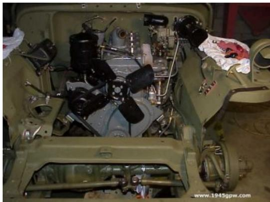
**REMOVE RADIATOR:** Remove the connections for the upper and lower tubes. There will be two bolts to remove on the bottom.
