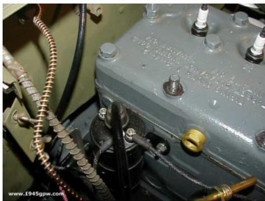
REMOVE COIL WIRE: this wire comes from the firewall, so you will need to remove it. As well as the cable to the distributor cap (if you take it off like I did.)
