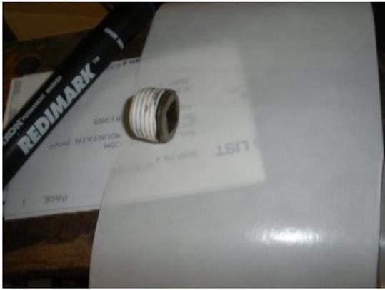
I will tape up all of the plugs around the transmission/transfer case to avoid dripping. If you changed the fluid then tighten this one back up and we will fill when we are on the passenger side.
