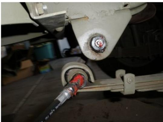
Moving around to the passenger side, grease the back spring shackles bolts
