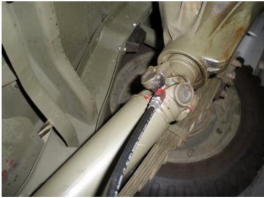
While under the jeep, shift to the back axle shaft and hit the zerk on the universal joint (if you can). If the zerk is not in a position, you will need to rotate by moving the jeep forward or backwards.
