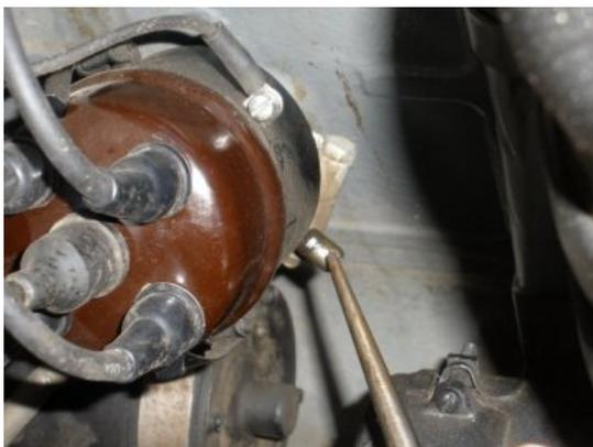
The last part of the lubing is the distributor oiler. If you have your oil can handy with oil in it, then move to your distributor and pull out your oiler and give it two drops of oil. Should be it! Now check your lubrication chart and check off all that you have done.
