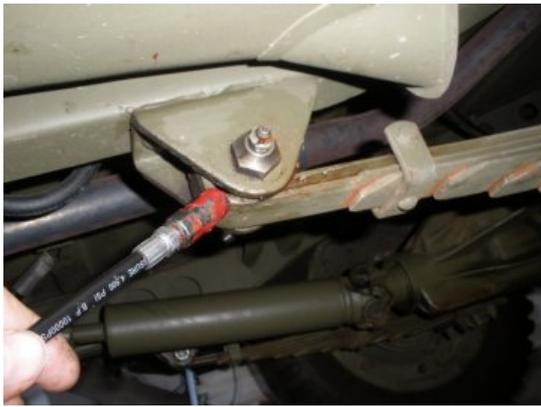
Next, scoot out from the jeep and hit the back wheel spring bolt. After this one is done, set the grease gun aside and check the fluids on the transmission
