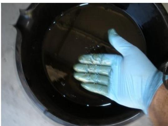
Now the last part. I drained my fluid on my transfer case side, so I need to replace that fluid. Before I do that, check the oil that was drained and check for metal fragments. If you find any have your transfer case checked by a professional. Otherwise your ok.
