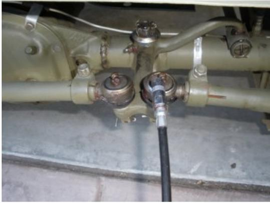
In the TM10-1513 I it also shows you the steps for lubing your vehicle. So between these steps and the manual from the link above you should be set to go. I start with the tie rods on the front of the jeep and move down the driver side and back around to the front on the passenger side. Here you see the two fittings for the Tie Rods, and I the third on the bell crank behind the tie rods.
