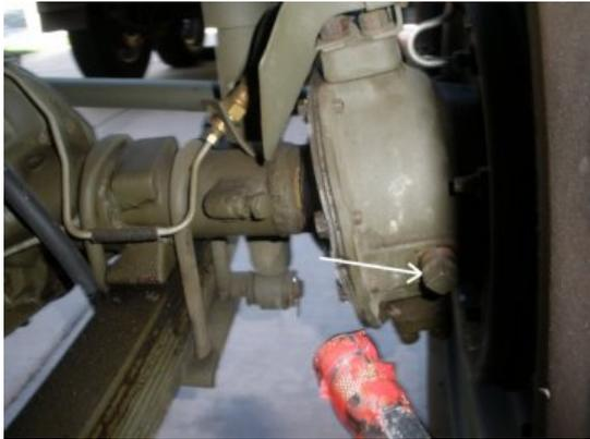
Remove the Front passenger axle plug and check your grease level. Give a few squirts if you find the level low.
