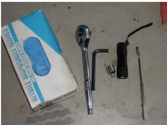
The second set of tools to have ready is the rubber gloves (it will be a little messy), a socket wrench for draining transmission gear fluid, a 3/8" allen wrench for transmission fill plug, and I always keep a magnetic pen ready, so when I drop my plug on the skid plate I can grab it quick.
