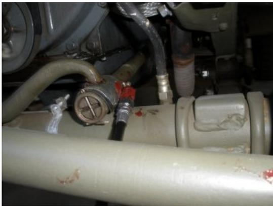
Behind the bell crank for steering is the drag link for steering. You can hit the front fitting while you are here. And get the back fitting when we are under the driver side.
