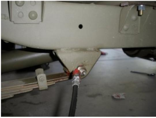
Move around the passenger back wheel and hit the rear spring shackle bolt.
