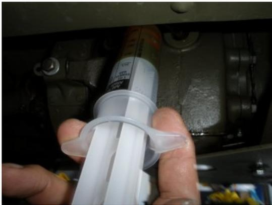
And I squirt the gear oil into the transfer case. With this device it takes about 5-6 fills to top off. But, no mess.
