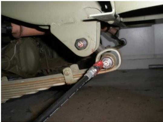
Now back to greasing fittings. On the driver side back spring shackle bolts get zapped both top and bottom.
