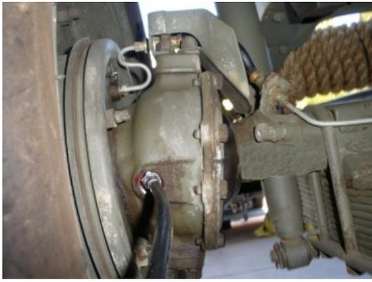
Next, unscrew the front axle universal plug behind the driver wheel. Stick your pinky finger into the axle housing and see if you can feel grease. Most likely not, as the grease settles at bottom. I will give 5-10 squirts into the drum.
