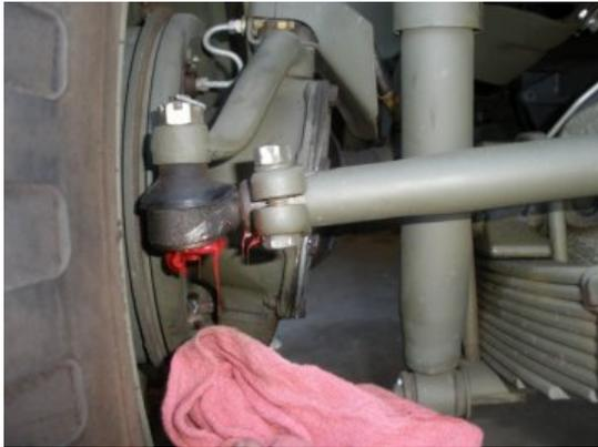
And last but not least, the front passenger side tie rod. Again, if you have a lot of grease, wipe it off. The more excess grease you have around the jeep the more grudge will collect. As you can see with these pictures, I need to go back and wash down from underneath.
