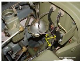
Install the horn wiring and mount the horn.
