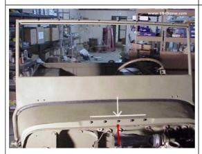
Install the hood to the five bolts on the tub, and the radiator stabilizer rod (in red) to the radiator.
