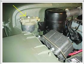
Early models with fuel strainer Install the fuel strainer to the the firewall of tub and connect the fuel lines to it.
