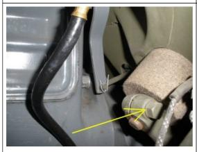
Install the brake and clutch pedals through tub floor the the armature, and secure. If you have the brake and clutch pads install them as well.
