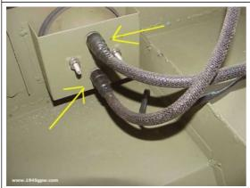
Install the wiring for the tail lights from the main harness (if not already), and finish up the wiring, battery, blackout lights, mirror, etc. At this point, you are pretty much done.
