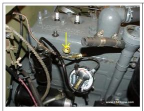
Install your temperature gauge line to engine block, and install the temp gauge in the dash.
