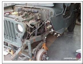
Install the front fenders to the tub and frame.
