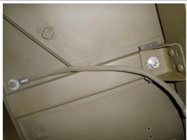
Install the ground strap from frame to the tub, and (not shown here), if you have a muffler out the passenger side (before late 44), then install the muffler clamp as well.
