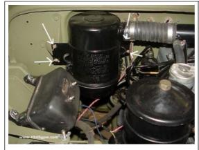
Install the air filter four wing nuts and connect the air tube hose to the air filter.
