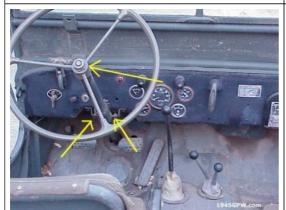
Install the steering column support, and steering wheel and nut.
