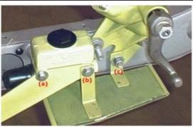
This picture with permission from Ed Campion shows in detail where each of the the bolts will be connected and the master cylinder positioned. From the top view there will be 3 bolts that are appart of this installation.
