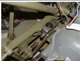
As you see in this last photo, the tie bar is connected to the brake/clutch tube, and the master cylinder is now protected by the heat shield.
