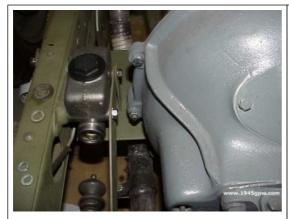
Now push the longer bolts through the tie bar and master cylinder. These bolts will lock into the frame.
