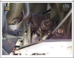
First you want to remove the wires by pulling them off of the terminal on the current switch. If you have a heat sheild installed, you are pressed for room and visibility is not that great.
