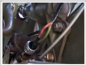
Hook the wires back up to the switch. Order does not matter. Be sure you feel a little "click" around the terminal when you install each wire.
