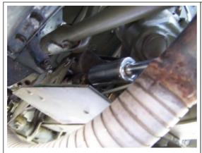
put the 1 inch socket around the old switch and crank it counter clockwise. It takes about a full turn before I can unscrew it with my hand.
