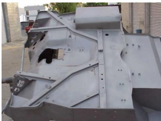
In addition, the clean surface allows you to inspect the metal for weaknesses. It was very easy to spot areas that I needed to replace due to weakness from rust or pitting. The surface is ready for welding as well!
