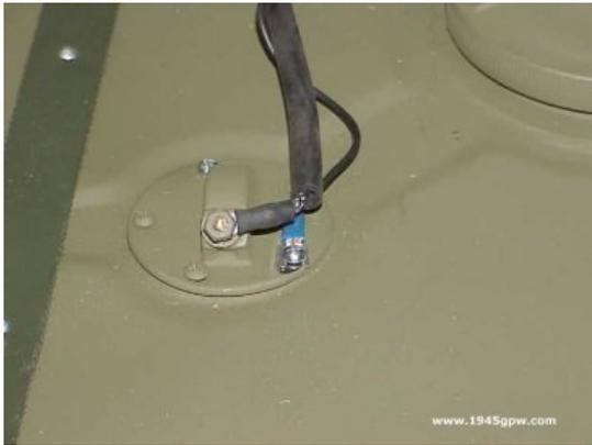
Before installing the straps, you can install the sending unit into the tank. Just drop the sending unit into the small hole on top of the tank and screw into the tank.
