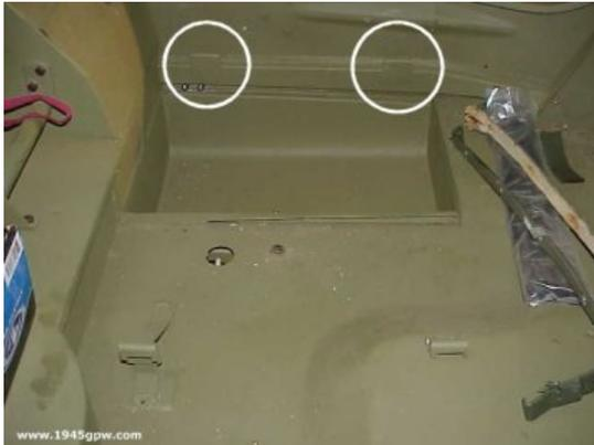
Installing the fuel tank is pretty easy, but the fuel tank straps can be difficult to find. Here we show you the empty tank well prior to the installing of the tank. Circled are the channel hooks that the straps will connect to.
