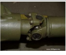
The installation of the ujoints is pretty basic once you get the cups installed on the clips side. Here you see it is a matter of tightening the U bolts on each side. Remember to keep the cups pressed on with your hand when installing. If they fall off, they will hit the ground and most likely fall out of place.
