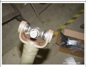
Here you see I have finished and the ujoint moves freely. Also, you see I removed the cups from the other direction. That way they don't fall on the ground while I was working with these two.
