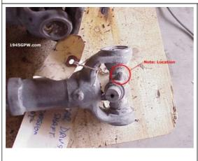
If you acquire a restoring project, you will most likely need to replace your u-joints. First, be sure you note where the location of your zerk fittings are (this picture shows the INCORRECT placement. the zerk should point toward the shafts). If you install these upside down they will be a bear to grease.
