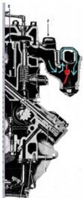
When the engine is cold, the counterweight will rest the valve flapper (red) in an open position, routing the warm exhaust air around the Fuel Intake manifold. Thus, help to vaporize the fuel as it is entering the carburetor. Light blue shows the direction of the exhaust when cold.
