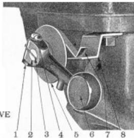
FIG. 2—HEAT CONTROL VALVE
