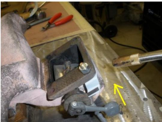
If the engine was running and warm, you would see the heat control valve move upward and the valve flapper would close on the inside of the manifold, diverting exhaust directly out the exhaust pipe. Interesting to note, after engine is warm, and you turn the engine off, you can watch the valve start to come down as the spring retracts and the counterweight force will open the valve up.
