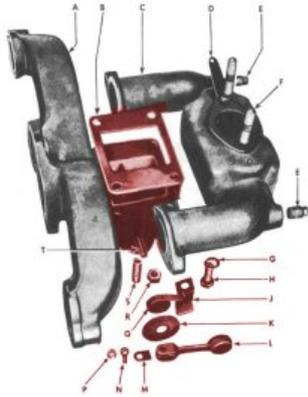
The Heat Control Valve, or Heat Riser on a WWII jeep was designed to help heat the intake air quickly in sever cold weather areas. Many jeep owners misunderstand the purpose of this component. First, the heat riser components that sit under the intake manifold and divert warm exhaust air. Components shown here.
