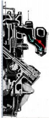
As the engine warms up, the circular spring will warm up and contract forcing the counterweight upward. This will close the valve and divert the exhaust straight out to the exhaust pipe.
