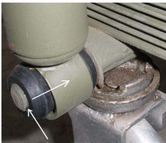
The previous picture shows us that we have enough room to push the washer and cotter pin on, but if you look at the bottom, we are going to need to compress the grommets in order to get the washer and cotter pin on. There is a specific tool to do this, but most of us don't have it, so we need to improvise.
