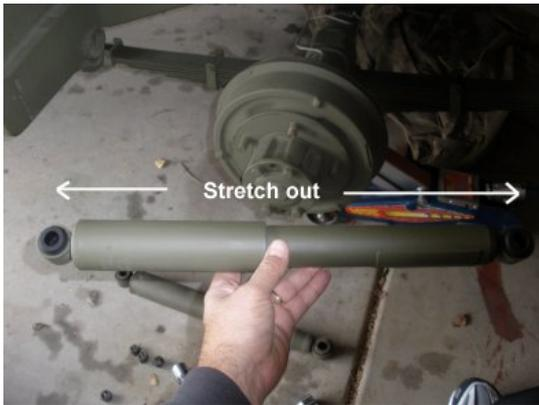
Next, pull the upper and lower legs of the shock and stretch them out. It is easier to compress the shock when adding to the frame than the latter.
