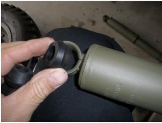
Next, prepare the shocks by placing the rubber grommets in both the upper and lower portion of the shock.
