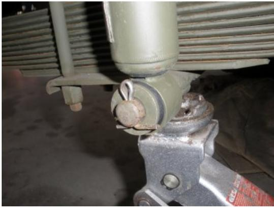
Now separate the cotter pin and the bottom is complete.
