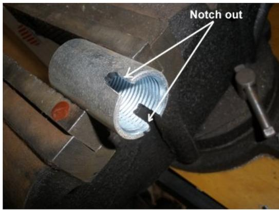
We found a little conduit coupling unit that fits over the pin of the bottom shock absorber. Because this piece is a \$1 piece, we are going to create a tool to help us compress the grommet. First, we notch out a section with a grinder, enough for the cotter pin to move around.
