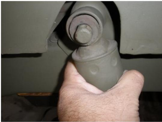
Next, wiggle the shock back and forth and the on the upper pin, and the shock will start to remove. Continue the same wiggle for the lower pin and the shock will pull off.
