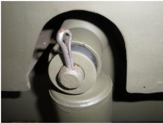
The upper section of the shock was a little better. In this case, was able to start the cotter pin, but the bottom of the pin was too tight.
