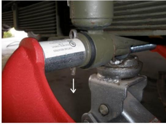
Once compressed enough, push the pin in. Note: you want to push the pin in as far as you can, because as soon as you release the C clamp the pressure on the cotter pin will not allow you to push it in any further.
