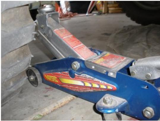
While replacing shocks may seem trivial, there can be some challenges getting the rubber bushings compressed in order to get the cotter pins on. While not necessary, we will take the wheel off in order to show you good pictures. First, we jack the rear driver wheel up.
