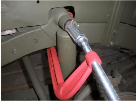
FRONT SHOCKS ?? The front bottom shocks can be applied like above, but what about the pesky top ? In this case, an 8 inch C clamp can work its way around the frame to apply the pressure needed to squeeze the grommets. **BE SURE** to do the top first on the front as well as back! Hope it helps!
