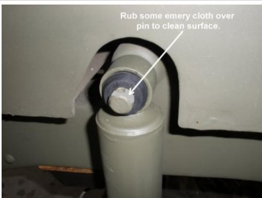
Use some emery cloth on the pins prior to pushing the shock/grommets on. Now, push both upper and lower legs of the shock on to the pins and push the grommets back to the frame as close as you can.
