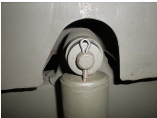
By pushing the bottom of the washer in, and tapping the cotter pin with a small hammer, the pin popped through (much easier than the bottom).
