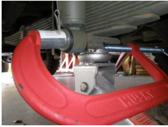
Next, we take an 8 inch C clamp and place the washer over the pin, with our modified coupling in place, and start compressing the clamp. Keep the C clamp straight and start compressing.
