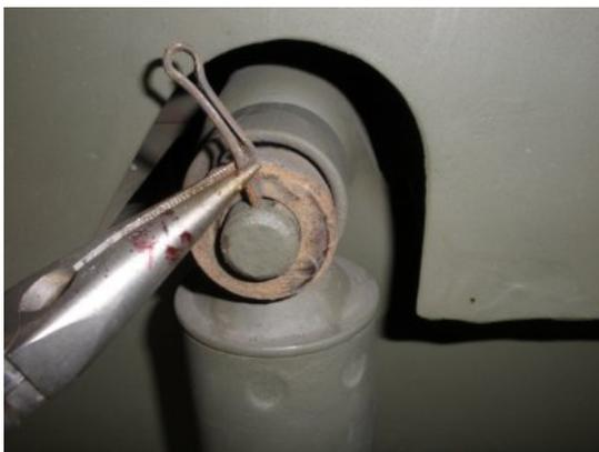
Straighten the cotter pin out on both the upper and lower areas and pull the cotter pin out.
